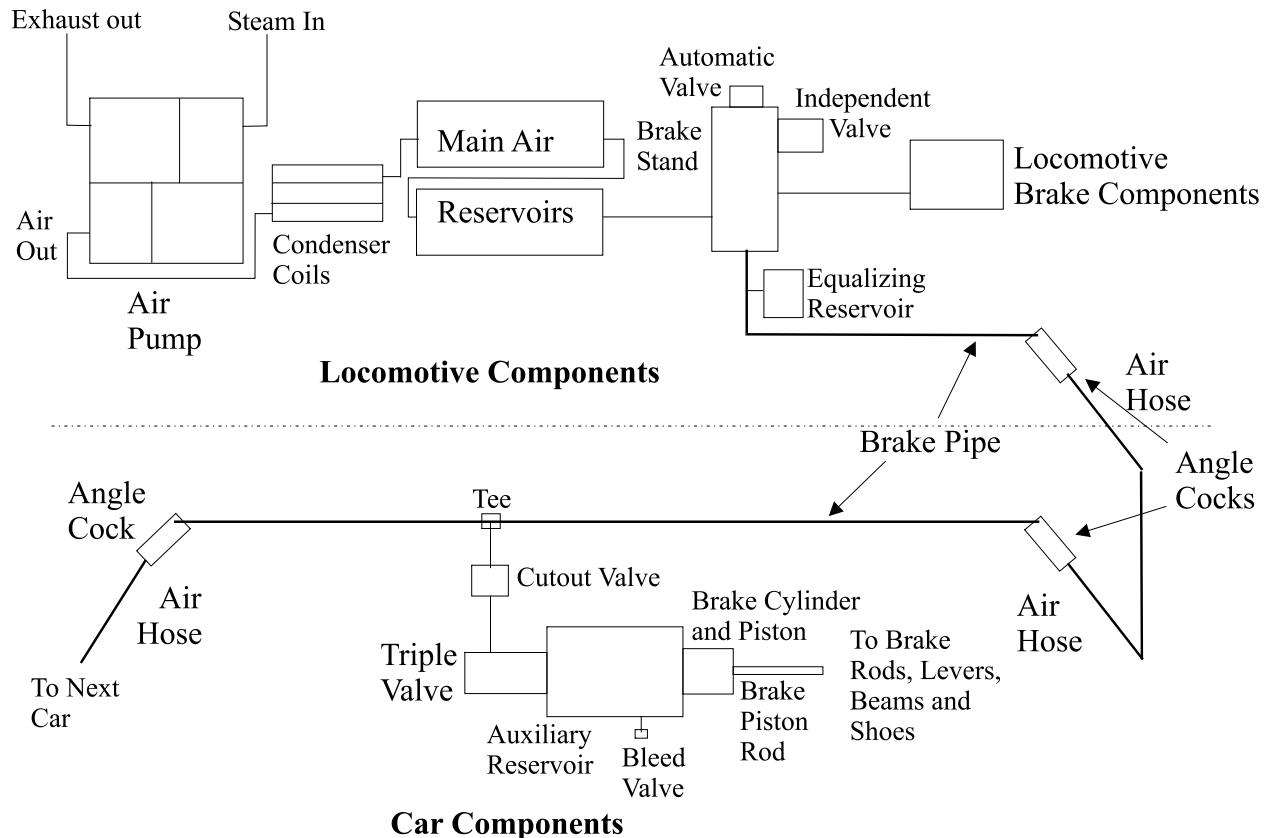
Emergency braking can be initiated at the locomotive Automatic Brake stand or by any crew member using a Conductor's Valve. Conductor Valves are located on cars throughout the train and are connected directly to the Brake Pipe. The Fireman also has access to an emergency valve. Once the brakes are set into emergency, the air may be completely exhausted from the Brake Pipe and the Conductor's Valves no longer have air, and therefore no longer function.
